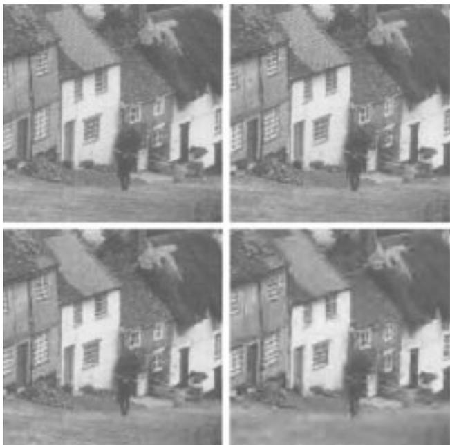
Fig. 12. Perceptual performances: Original “Goldhill” (upper left), PSNR = 31.73 dB at 0.41 bpp (upper right), PSNR = 29.94 dB at 0.24 bpp (lower left), PSNR = 27.42 dB at 0.1 bpp (lower right).
