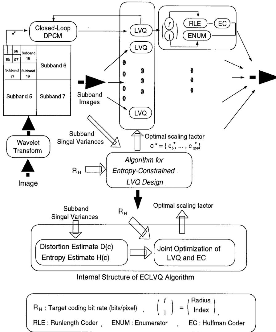
Fig. 8. Wavelet-based image coding system with entropy constrained LVQ designed by proposed algorithm.
