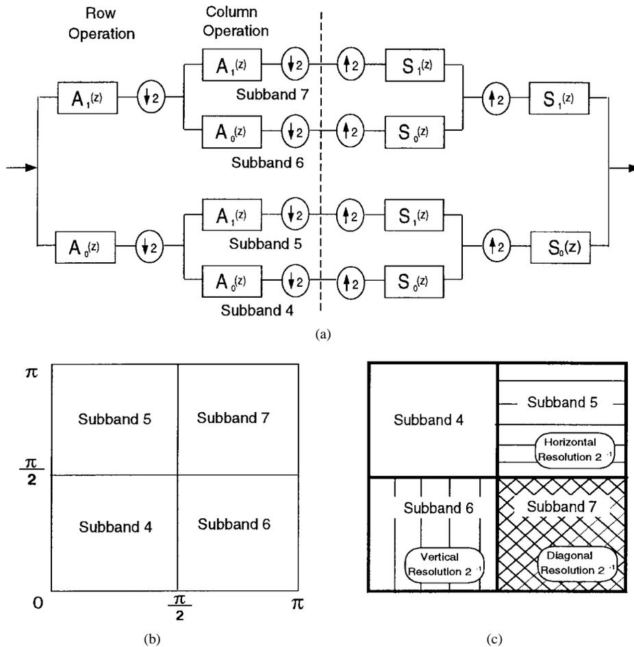
Fig. 1. (a) A tree-structured connections of separable two-dimensional QMF's, (b) its subband decomposition map, and (c) multiresolution map. The leaf node set of this wavelet tree is  $L(S) = \{4, 5, 6, 7\}$ .
