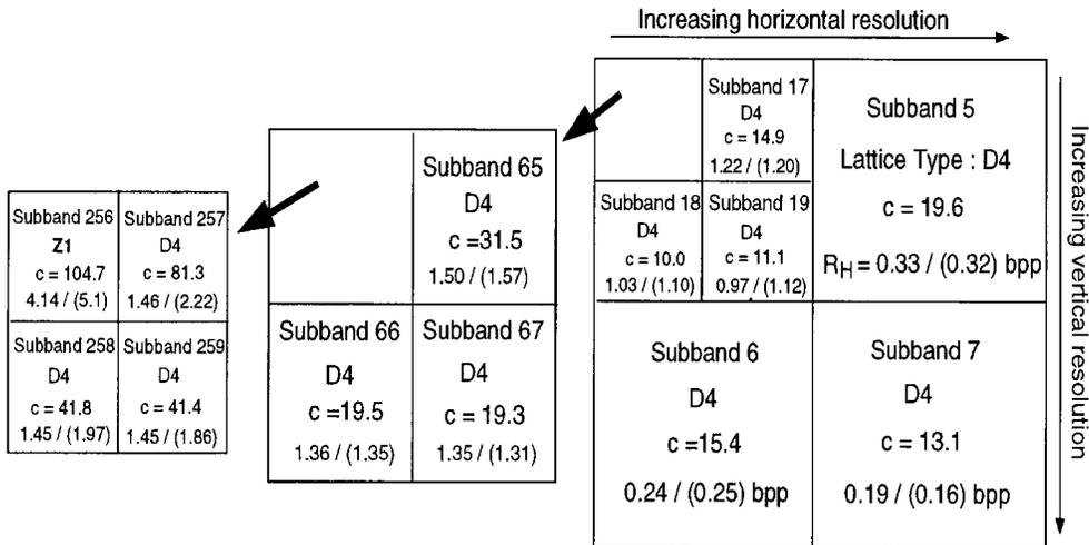
Fig. 9. 0.5 bits/pixel coding strategy for "Lena."  $c$  is the estimated optimal scaling factors at each subband.  $R_H$  is allocated entropy rate. The bit rate in parenthesis is actually obtained from binary file.
