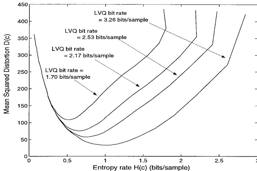
Fig. 6. Distortion versus Entropy curves for various LVQ bit rates. The test data is subband 17 (*lllh*) of  $512 \times 512$  "Lena."
