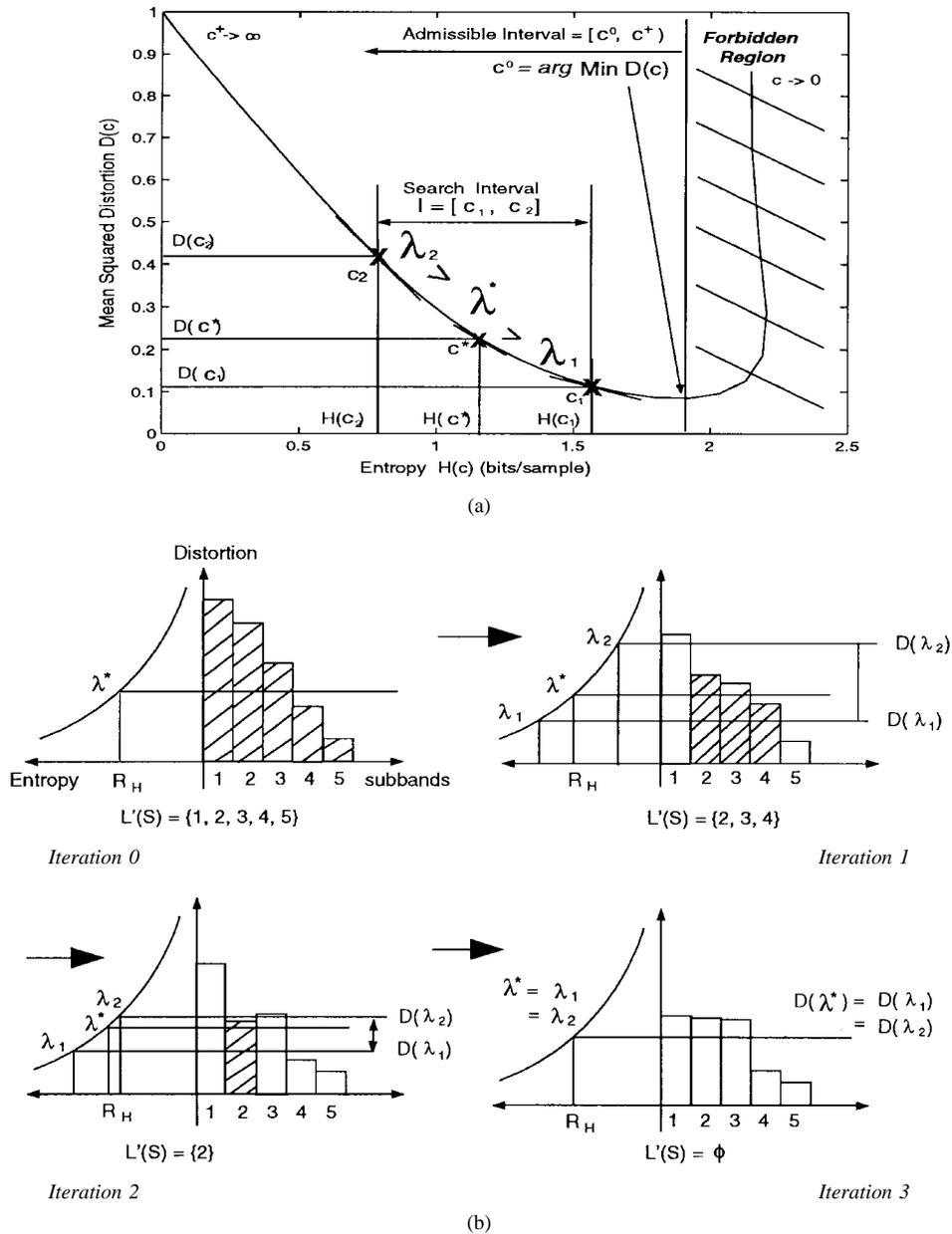
Fig. 7. (a) Search procedure for the optimal scaling factor  $c^*$  at a subband and (b) entropy allocation procedure.
