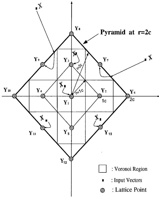
Fig. 2. Pyramidal lattice vector quantization scheme for two-dimensional cubic ( $Z^2$ ) lattice.  $B^{gr}(2c) = \{X: \|X\|_1 \leq 2c\}$ ,  $B^{ov}(2c) = \{X: \|X\|_1 > 2c\}$ .  $C = \{Y_1, Y_2, \dots, Y_{13}\}$ , code radius  $m = 2$ , code size  $|C| = 13$ , bit rate  $R = \log_2 |C|/\text{dimension} = 1.85$  bit/sample, lattice points on pyramid:  $C_s(0) = 1$ ,  $C_s(1) = 4$ ,  $C_s(2) = 8$ .
