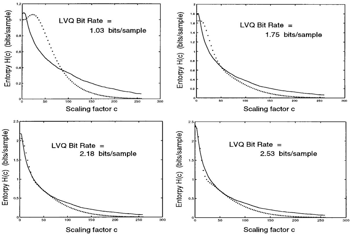
Fig. 4. Real entropy (solid line) and estimated entropy (dotted line) for subband 17 (*llh*) of  $512 \times 512$  “Lena.” Lattice type is  $D_4$ . The vector size is  $N = 4096$ .
